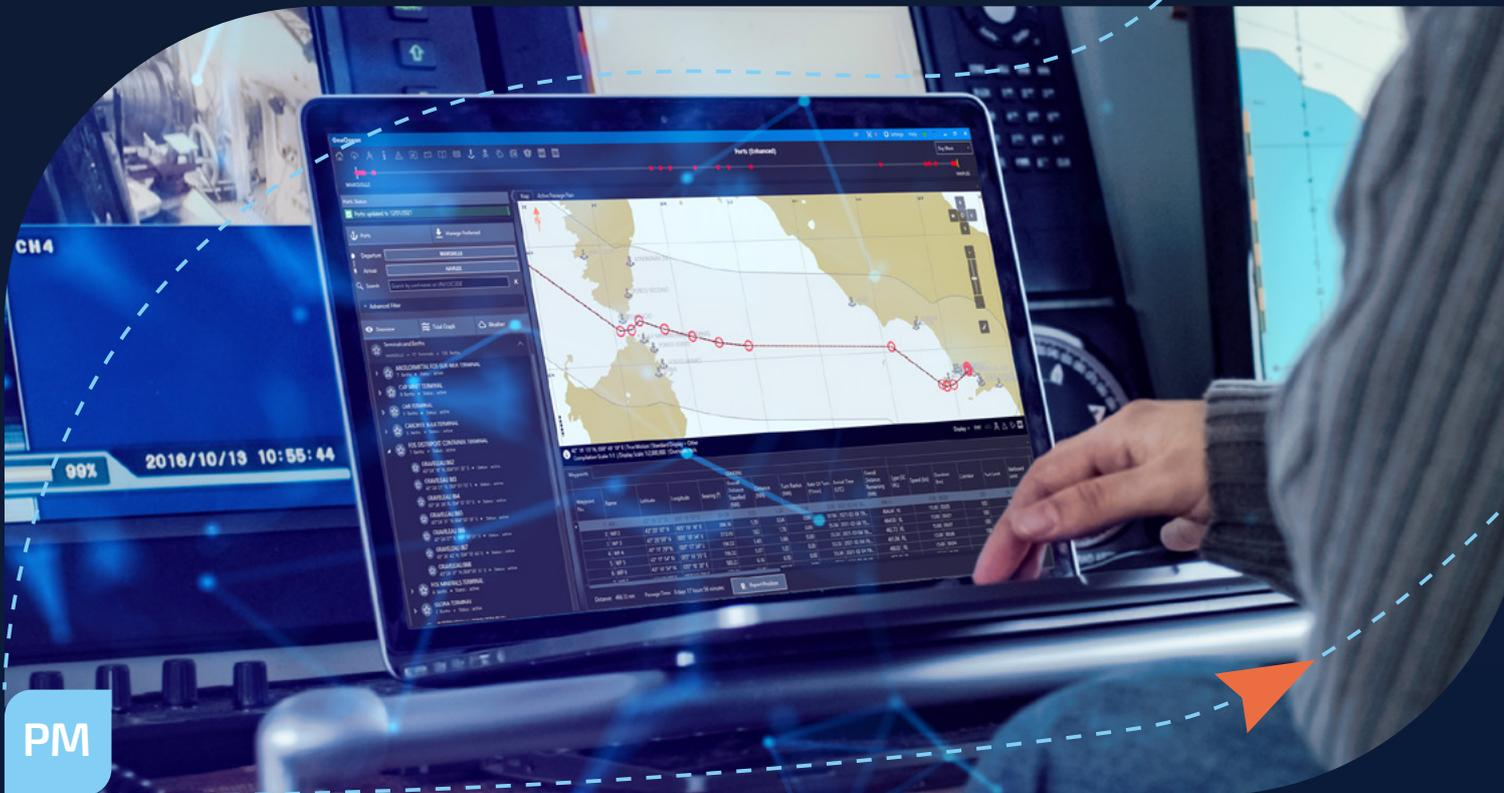
PassageManager utilises port, route, tidal and weather data to create a comprehensive and fully customised digital passage plan within minutes. To ensure route accuracy users enter detailed information about their vessel, including its equipment, characteristics, ship parameters, UKC limits, weather thresholds and more.
